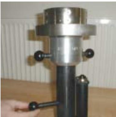
4. The expansion insert must be removed for the pressing operation. To do this, remove the long guide pin and pull the short guide pins out as far as the limit stop.
