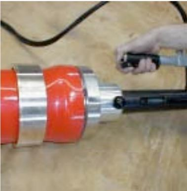
4. The time that the fitting is inserted in the pipe can be influenced by maintaining the expansion pressure with the expansion head fully opened (final position in the expansion procedure).
