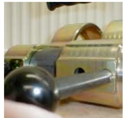
9. The second position is the final position so that the sliding sleeve can be pushed up flush with the fitting collar (final position).
