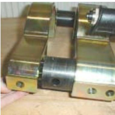
7. First push on the long frame press, and then the short one, and insert the long guide pins completely. Check that the frame sets are aligned correctly (the short fixed frame is flush with the edge of the cylinder)!
