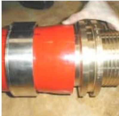
5. Insert the fitting into the pipe. After a short time, the fitting stays in a fixed position in the pipe (memory effect).
