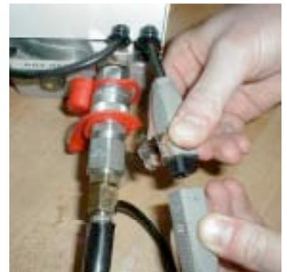
6. The control cable for the "master cylinder" must be connected to the unit.
