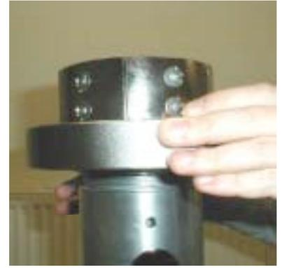
3. Expansion heads 125 and 160 are screwed directly onto the expansion insert. To do this, the heads must be applied so that they are flat, and must be completely screwed on.
