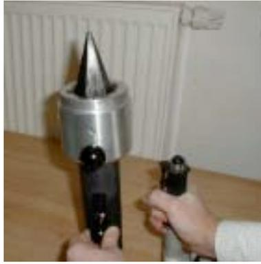
2. The expansion insert is introduced all the way into the cylinder and is fixed with the 2 short guide pins and the long guide pin. Caution! Insert the guide pins completely!
