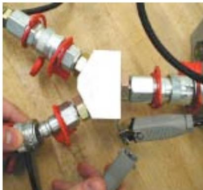
5. For the pressing operation, both cylinders must be connected to the unit via Y-distributors (rapid-action connector on hydraulic hose or unit)
