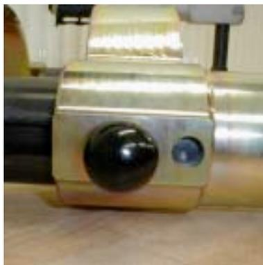
8. The long (movable) frame has 2 guide pin positions. The first one is the starting position, when the sliding sleeve is still a long way from the fitting collar.
