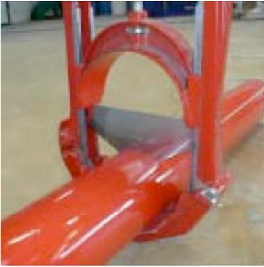
1. Cut the pipe to the desired length, at right angles, using the guillotine (article number 249340).
